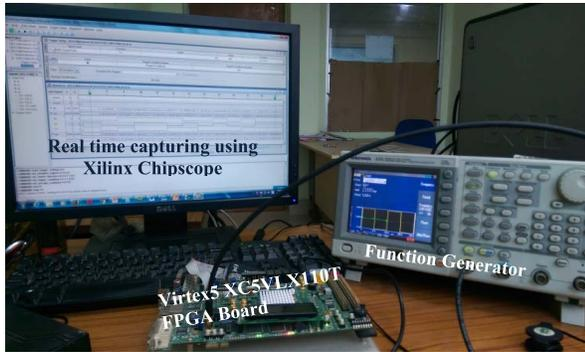
Fig. 8. Laboratory experimental setup of the proposed architecture of the modified dual-CLCG method of 32-bit word size.
