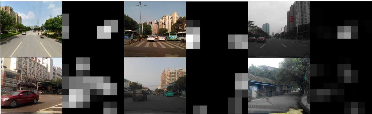
Fig. 9: Test examples by the GoogleNet. For each image we display its groundtruth-labels. Gray images on their right side are feature maps generated by the resolution-adapted layer, with bright pixels to indicate greater weights.
